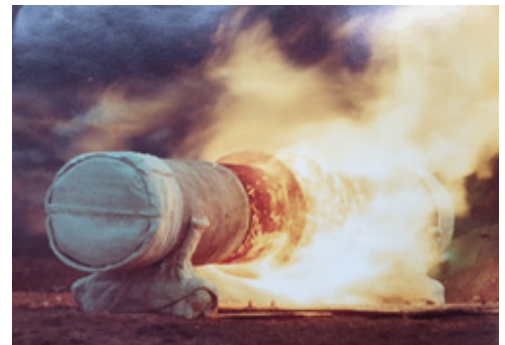
Photo courtesy Tom Royle: Jet fire test on riser protection system at Spadeadam
