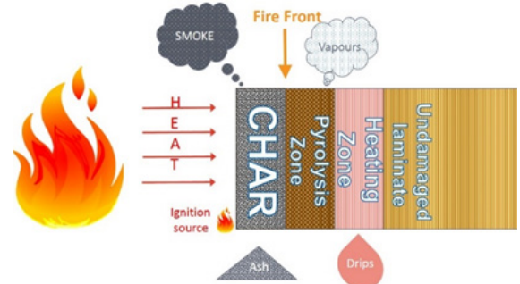
Progression of fire within a composite, courtesy of Nigel Keen.
