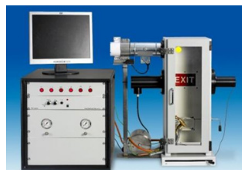
Photo courtesy Fire Testing Technology: ASTM D2843 Smoke Density Test Rig
