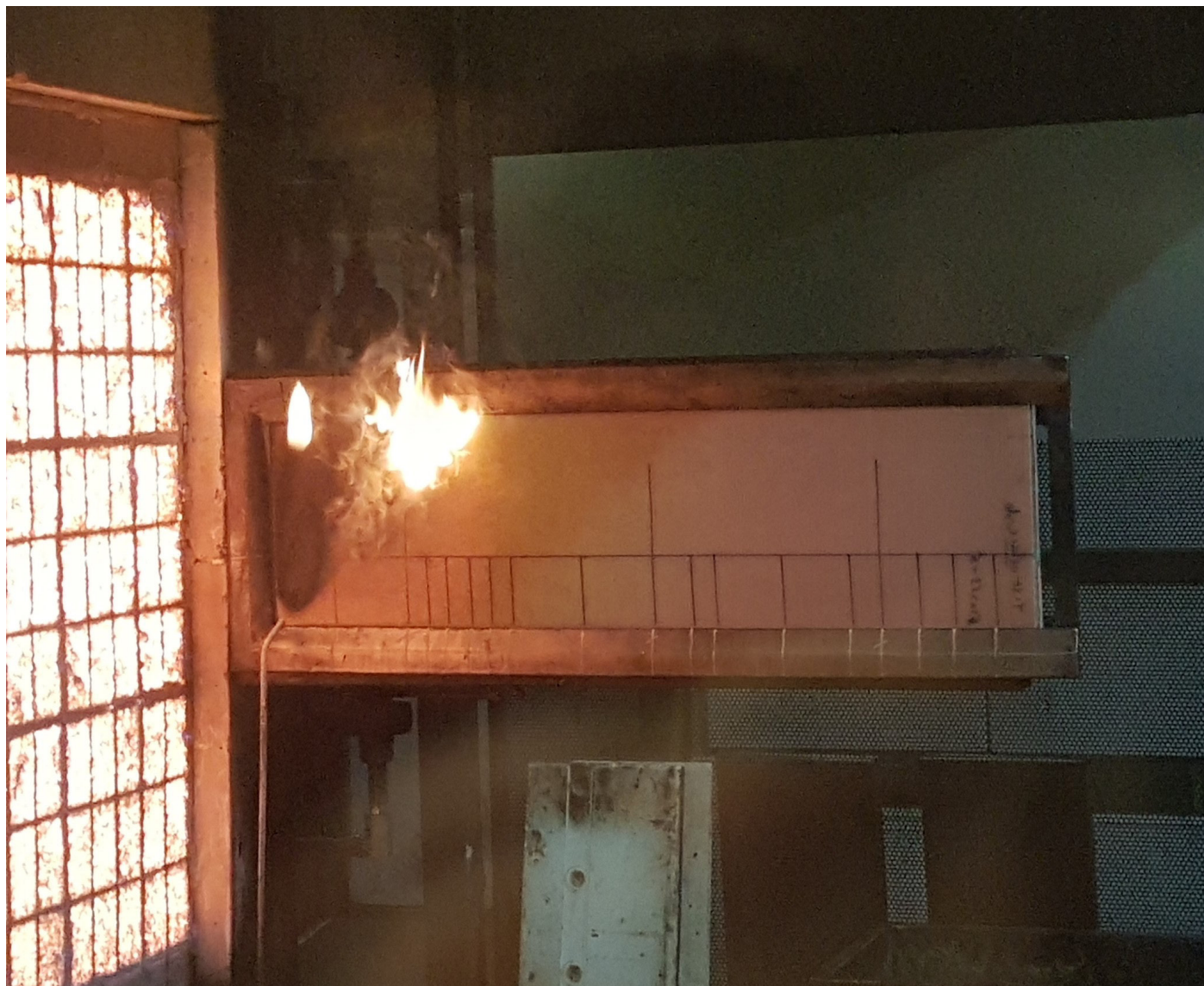
Figure 4: Filon G104 GFRP rooflight sheet achieves Class 1 to BS 476 Part 7 for surface spread of flame. Photo courtesy of Filon Products Ltd.
