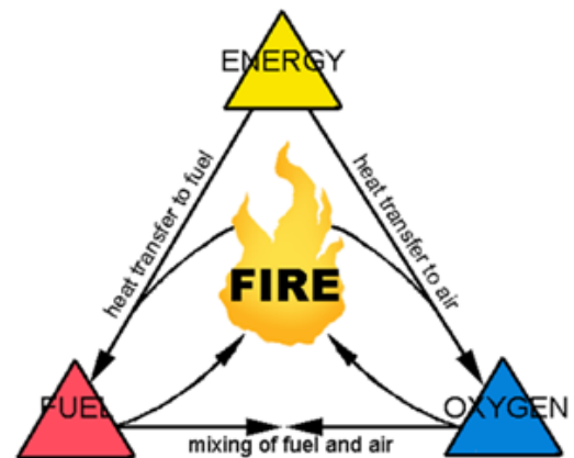
Fire triangle, courtesy of Nigel Keen.
