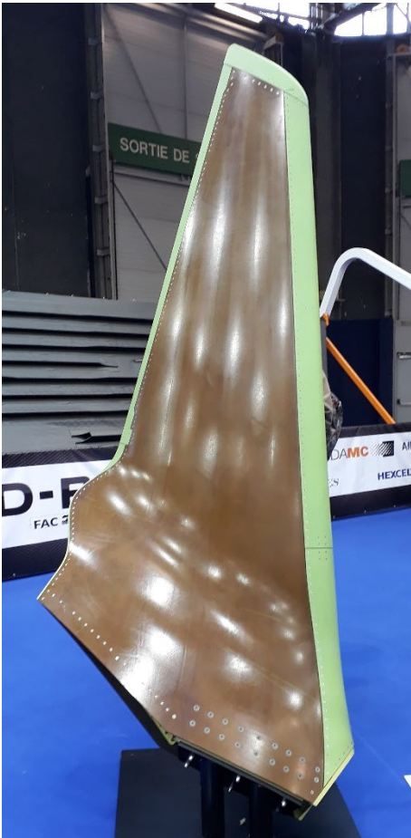
Figure 14: Composite tailplane structure showing mechanical fasteners. Photo: Composites UK
