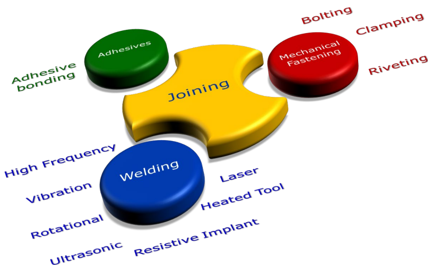
Figure 4: Summary of a selection of joining processes: bonding, welding and fastening
